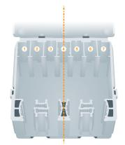
The Wagobox-XLA is designed to support either one or two circuits that can be supplied together or separately. It is important to ensure that this is indicated on the lid using permanent marker or labels.
