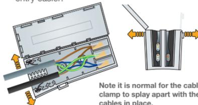
**Note** it is normal for the cable clamp to splay apart with the cables in place.
